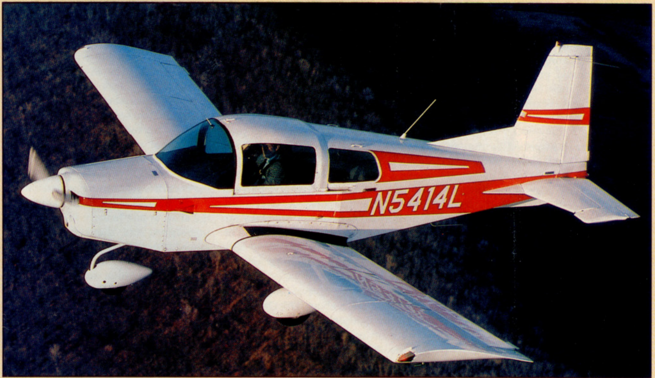
Smooth, bonded skins help early "blunt nose" Travelers coax respectable speed from 150 horses.
